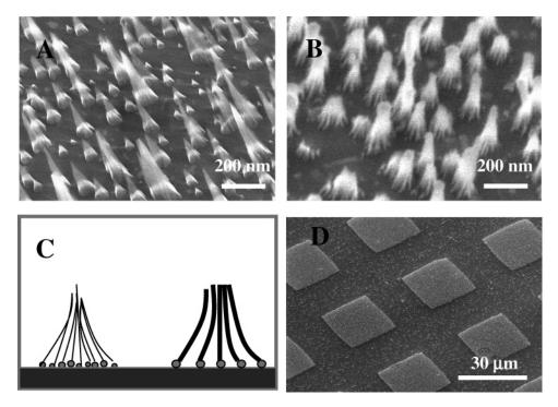
**Figure 1.** SEM images of BNNT bundles grown at a substrate bias of (A) -380 V and (B) -450 V and (C) their corresponding bundling configurations (left and right, respectively). (D) Patterned growth of BNNTs.
