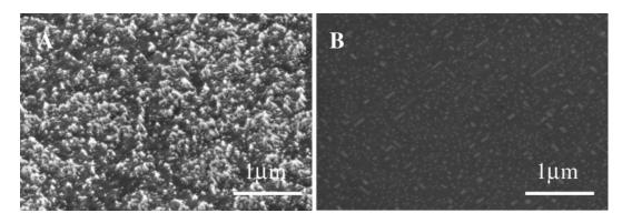
**Figure 4.** (A) SEM image of a sample deposited at low substrate bias (-300 V). Iron particles coated with BN films are detected. (B) SEM image of sample prepared without the deposition of boron nitride plume (simply plasma treatment at substrate bias of -400 V). Most Fe particles are sputtered away.
