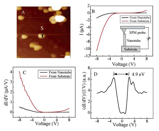
**Figure 5.** (A) AFM images of the vertically aligned BNNT bundles. T and S representing BNNTs and substrate surface, respectively. (B) I/V curve obtained from point T (back curve) and S (red curve). Inset shows the related measurement setup. (C) dI/dV curves obtained from the point T (black curve) and S (red curve). (D) Normalized differential conductance for BNNTs representing their LDOS and a band gap of ~4.9 eV.
