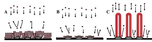
Figure 3. Schematic drawing representing the growth region of BNNTs. (A) Deposition of BN films on Fe nanoparticles due to low resputtering rate of the growth species. (B) Reduced growth rate of BN films from energetic growth species. (C) Total resputtering region where BNNTs are grown and BN films are suppressed.
