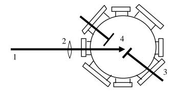
*Figure 1S.* Schematic of the PE-PLD system. Laser beam (1) is focused by a lens (2) on a rotating BN target (3). The BN growth specie from the target will be accelerated toward the substrate (4) by the substrate bias
