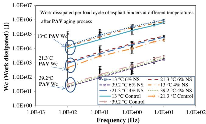
**Fig. 9.** Work dissipated per load cycle of control and nanosilica modified asphalt binder after PAV aging process (fatigue cracking influence, with standard error bars)
