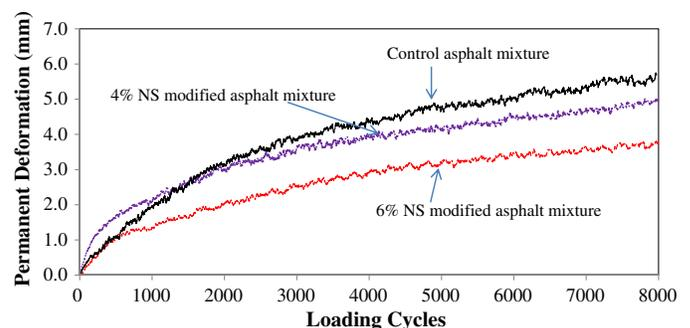
**Fig. 15.** APA rutting results of control and nanosilica modified asphalt mixtures
