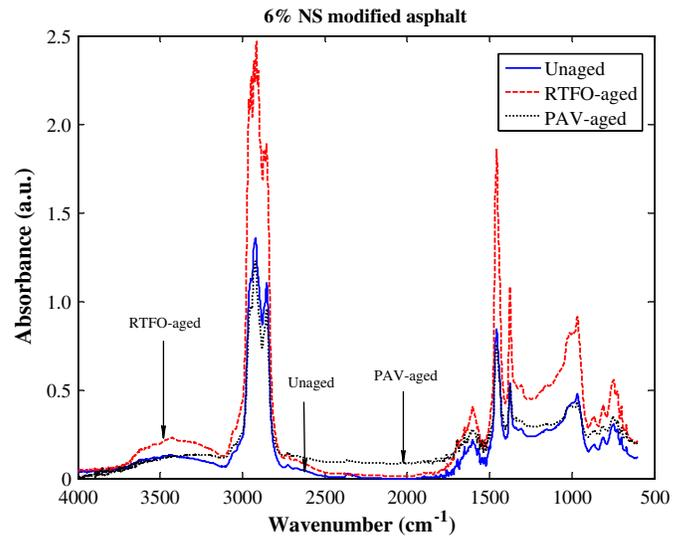
Fig. 13. FTIR spectra analysis of 6% nanosilica modified asphalt binder
