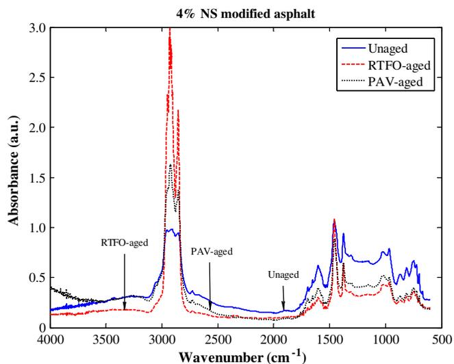
Fig. 12. FTIR spectra analysis of 4% nanosilica modified asphalt binder
