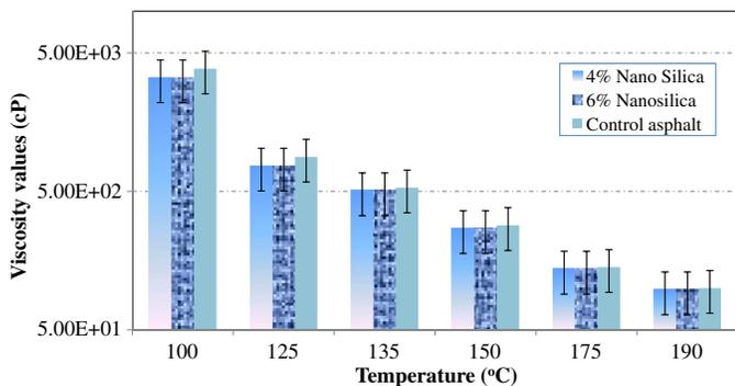
Fig. 3. Viscosity values of control and nanosilica modified asphalt binder
