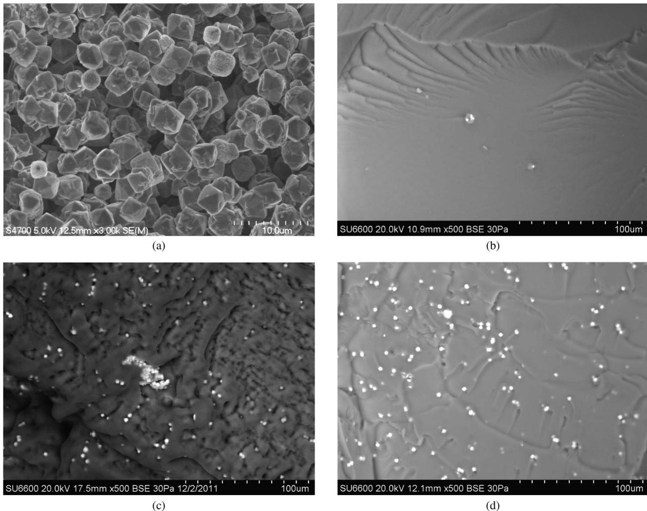
**Fig. 1.** FE-SEM microstructure images of nanosilica, control and nanosilica modified asphalt; (a) SEM image of nanosilica at 3,000× magnification; (b) SEM image of control asphalt binder at 500× magnification; (c) SEM image of 4% nanosilica modified asphalt binder at 500× magnification; (d) SEM image of 6% nanosilica modified asphalt binder at 500x magnification
