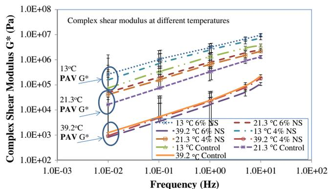
**Fig. 8.** Complex shear modulus  $G^*$  of control and nanosilica modified asphalt binder after PAV aging process (with standard error bars)
