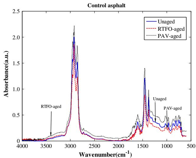
Fig. 11. FTIR spectra analysis of control asphalt binder
