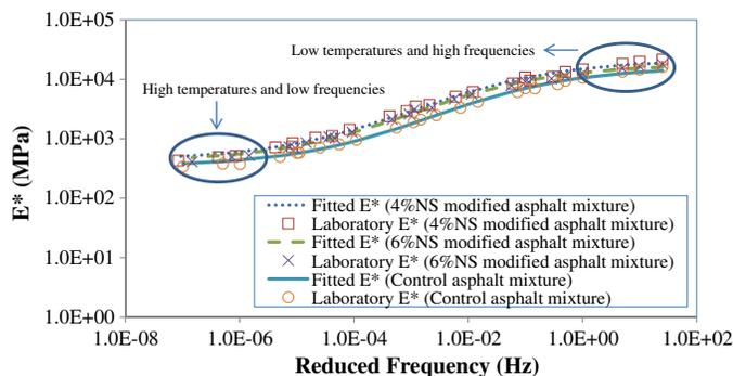
**Fig. 14.** Dynamic modulus results of control and nanosilica modified asphalt mixtures
