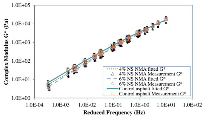
Fig. 4. Complex shear modulus ( $G^*$ ) master curves of nanosilica modified asphalt binder and control asphalt binder (with standard error bars)
