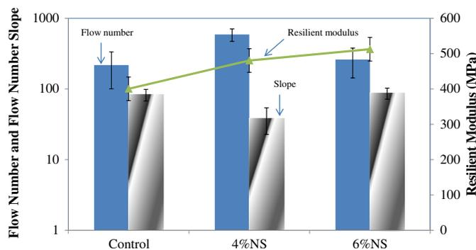
**Fig. 16.** Flow number results of control and nanosilica modified asphalt mixtures
