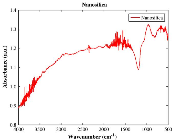
Fig. 2. FTIR spectra analysis of nanosilica
