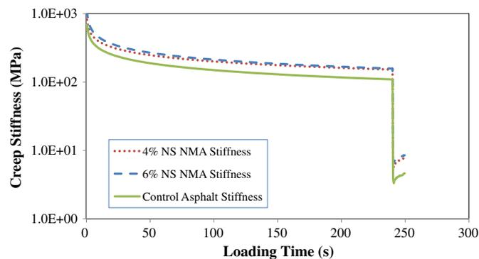
**Fig. 10.** Creep stiffness of control and nanosilica modified asphalt binder in BBR test
