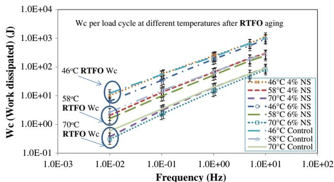
**Fig. 7.** Work dissipated per load cycle of control and nanosilica modified asphalt binder after RTFO aging process (rutting influence, with standard error bars)
