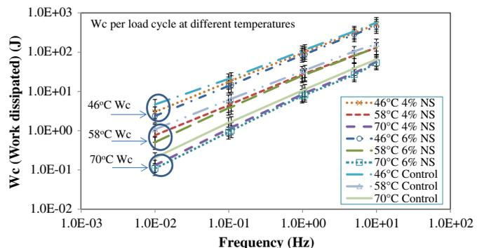
Fig. 5. Work dissipated per load cycle of nanosilica modified asphalt binder and control asphalt binder (rutting influence, with standard error bars)
