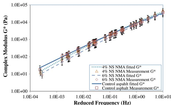
**Fig. 6.** Complex shear modulus ( $|G^*|$ ) master curves of control and nanosilica modified asphalt binder after RTFO aging process (with standard error bars)
