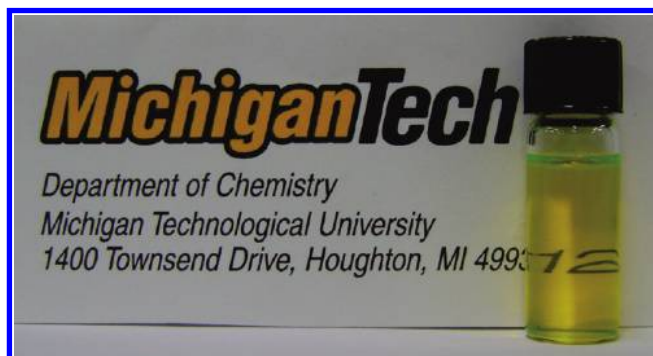
FIGURE 2. Digital photo picture of composite solution of BNNTs and polymer A in \text{CHCl}_3 .
