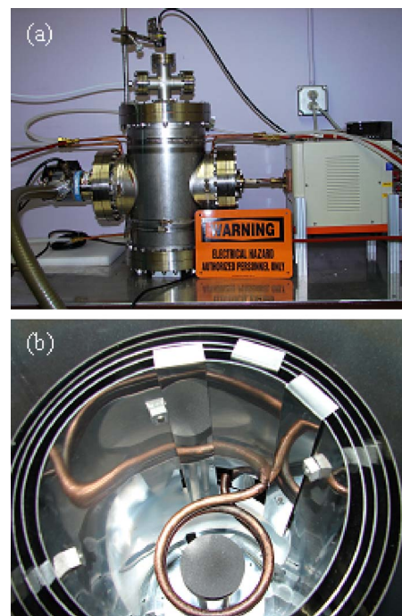
FIG. 2. (Color online) (a) The exterior view and (b) the interior view of the induction chamber.
