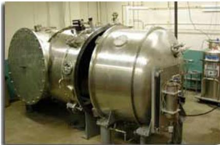
**Figure 1.** Space simulation chamber at Michigan Tech used for the erosion test.
