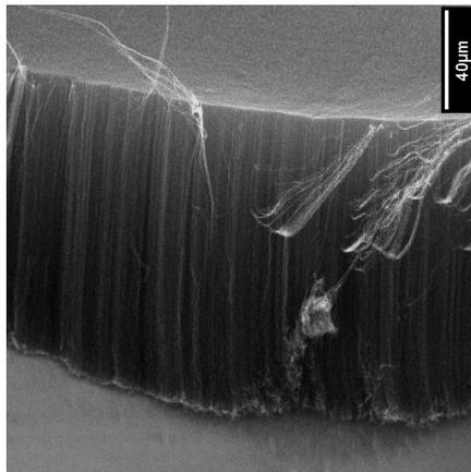
**Figure 3.** High-density vertically aligned MWNTs grown from  $C_2H_2 / Ar$  gas mixture for 15 minutes.
