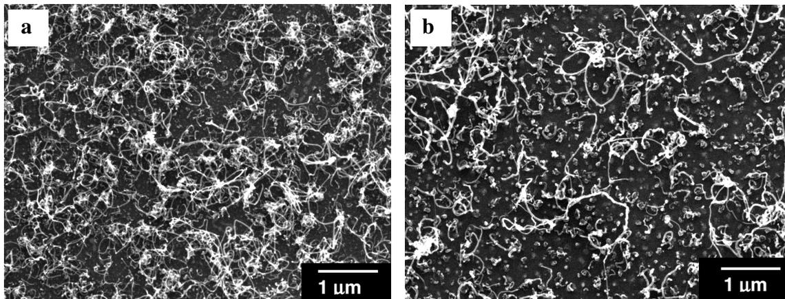
**Figure 2.** MWNTs grown from (a) pure  $C_2H_2 / H_2$ , and (b)  $C_2H_2 / N_2$  mixed gases.
