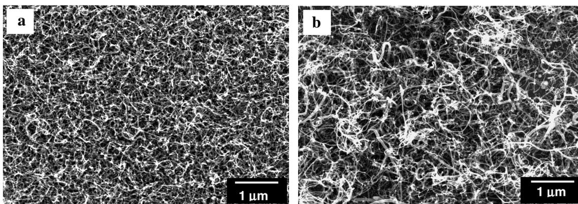
**Figure 1.** MWNTs grown from (a) pure  $C_2H_2$  gas and (b)  $C_2H_2$  / Ar mixed gas.
