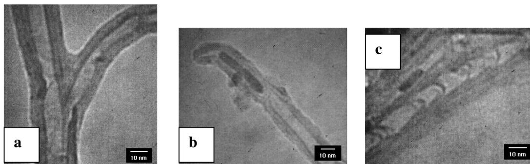
**Figure 4.** (a) Branching, (b) dome-capped, and (c) bamboo-like MWNTs.
