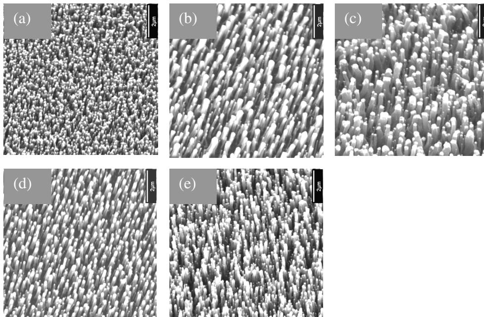
**Figure 3.** SEM images of VA-MWNTs grown at different substrate bias voltages as controlled by the bottom plasma (a)  $-50$  V, (b)  $-100$  V, (c)  $-150$  V, (d)  $-200$  V, and (e)  $-250$  V. Other growth parameters remained constant.
