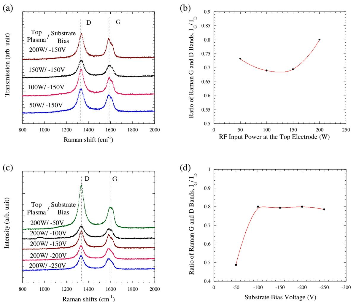
**Figure 4.** (a) Raman spectra for VA-MWNTs grown at various top plasma forward power and (b) the corresponding  $I_G/I_D$  relation. (c) Raman spectra for VA-MWNTs grown at various substrate biasing and (d) the corresponding  $I_G/I_D$  relation.
