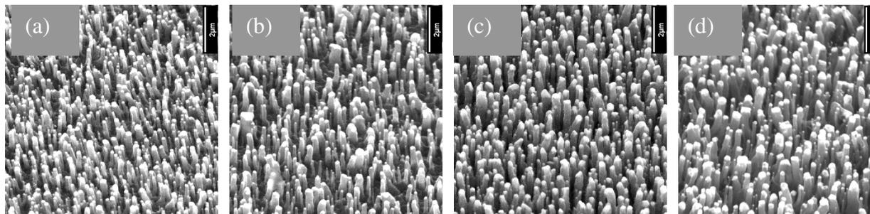
**Figure 2.** SEM images of VA-MWNTs grown at different top plasma forward powers (a) 50 W, (b) 100 W, (c) 150 W, (d) 200 W. Other growth parameters remained constant.
