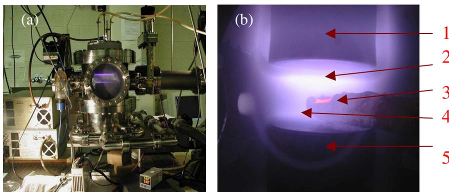
**Figure 1.** (a) Experimental setup of the dual RF-PECVD chamber. (b) Magnified view of (1) top electrode (2) top plasma (3) heater (with substrate) (4) bottom plasma (5) bottom electrode
