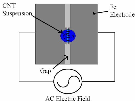
**Figure 1.** The DEP experimental setup. An AC electric field is applied between Fe electrodes before a CNT suspension is dropped into the gap. The field is left on until the drop is completely dry.
