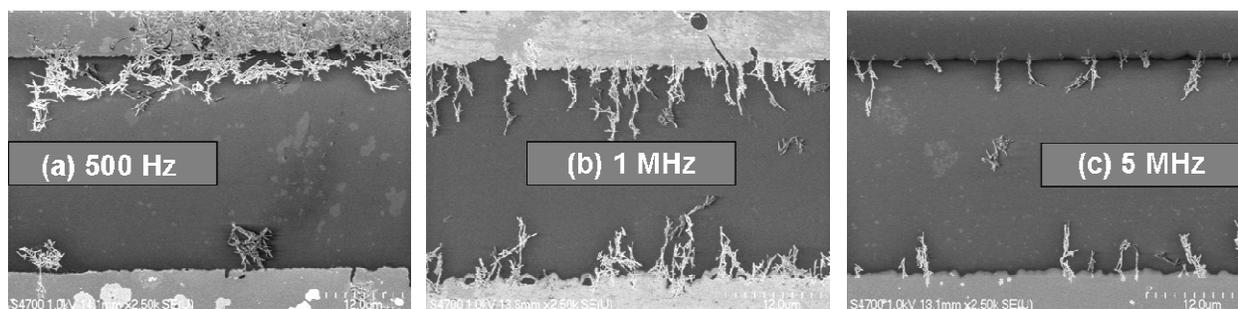
**Figure 4.** SEM images of PECVD grown CNTs subjected to an applied AC field of  $V = 20 V_{pp}$  at varying frequencies: (a)  $f = 500 \text{ Hz}$ , (b) 1 MHz, (c) 5 MHz. Gap distance  $\sim 25 \mu\text{m}$ .
