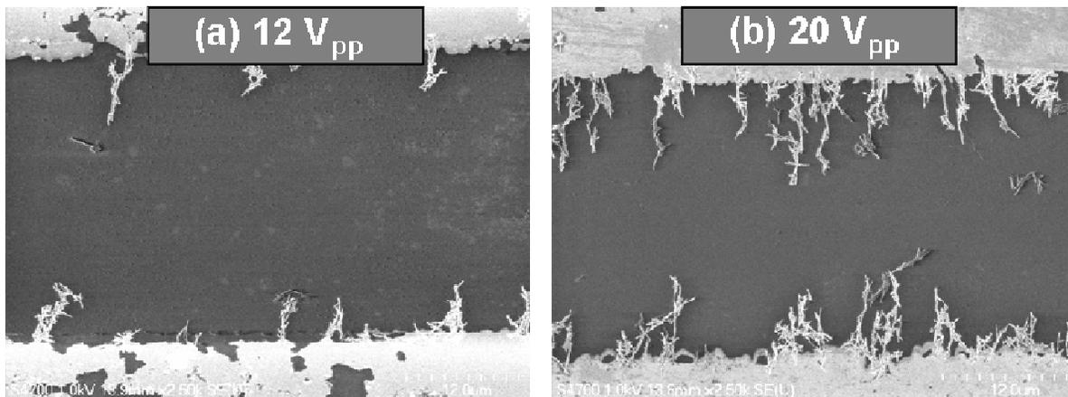
**Figure 3.** SEM images of PECVD grown CNTs subjected to AC fields with 1 MHz frequencies, but varying field strengths: (a)  $V = 12V_{pp}$ , (b)  $V = 20V_{pp}$ . Gap distance  $\sim 25 \mu\text{m}$ .
