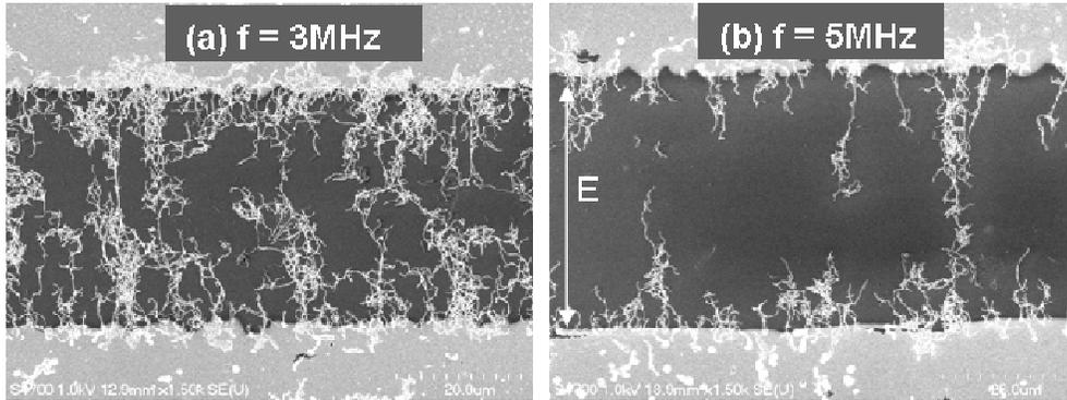
**Figure 5.** Thermal CVD grown CNTs, dispersed with 20 V<sub>pp</sub> applied. Increasing the frequency of the AC field shows a reduction in tube density from 3 MHz (a) to 5 MHz (b). Gap distance ~ 30 μm.
