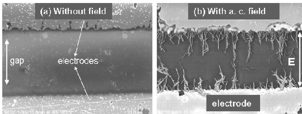
**Figure 2.** SEM showing the effects of AC fields on orientation of CNTs. (a) Tubes deposited with no field. (b) Tubes deposited with a  $V = 10 V_{pp}$  and 5 MHz AC electric field. Gap distance  $\sim 25 \mu\text{m}$ .
